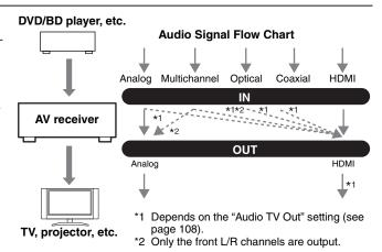
If signals are present at more than one input, the inputs will be selected automatically in the following order of priority: HDMI, digital, analog.
